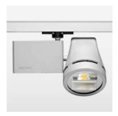
Spotlight for LED arrays, active cooling, reflector with double asymmetrical light distribution pattern, 99.99% pure aluminium reflector made of MIRO-SILVER®, pivoted emitter, adjustable luminaire head, die cast aluminium luminaire housing, powdercoated, multiadapter, driver unit, 220-240 V, 50/60 Hz
